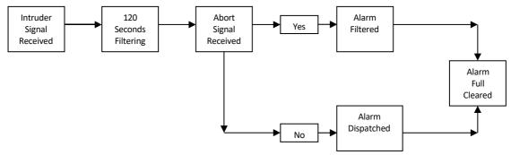
If the alarm activates during setting or un-setting, the system must be turned off within one hundred and twenty seconds to automatically abort the activation. There is no need for the End User to ring the ARC/RVRC.
